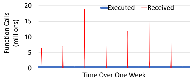
Figure 4. The load of a spiky function. This function allows its function calls to be executed with a 24-hour SLO. XFaaS leverages this property to spread out its function execution.
