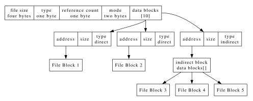
The size of the inode is constrained so that an even number of inodes fit into each block (inodes won't span blocks). The inode does not identify itself; if you need to manipulate an inode, the number is a necessary identifier; the cached inode itself will not have enough information to write it back to disk in the right place.
