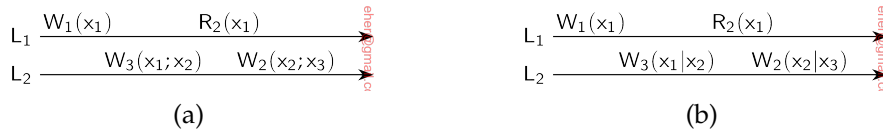
Figure 7.21: (a) A writes-follows-reads consistent data store. (b) A data store that does not provide writes-follows-reads consistency.
