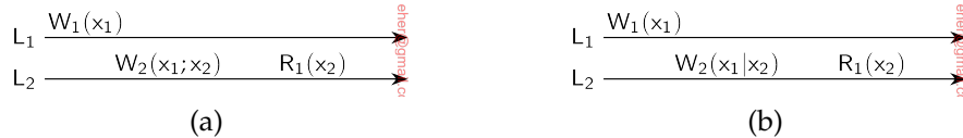
Figure 7.20: (a) A data store that provides read-your-writes consistency. (b) A data store that does not.
