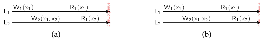
Figure 7.18: The read operations performed by a single process P at two different local copies of the same data store. (a) A monotonic-read consistent data store. (b) A data store that does not provide monotonic reads.
